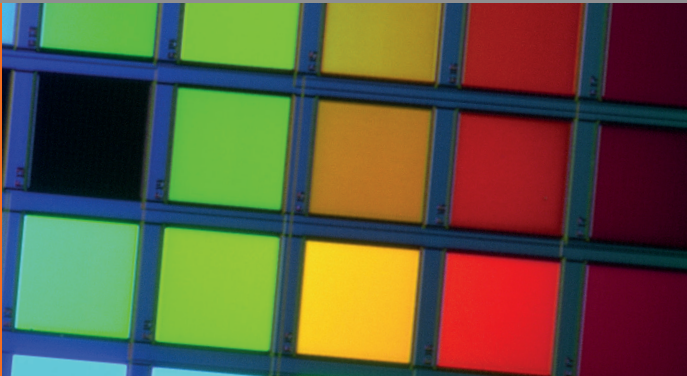
1 Microscope image of a color sensor chip
